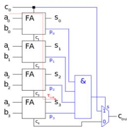
Fig -3: 4-Bit Carry Skip Adder
