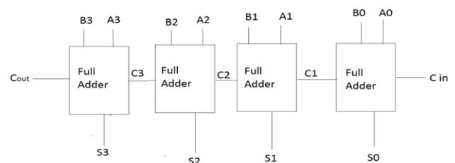
**Fig -1:** (RCA) Ripple Carry Adder
